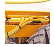
Admixture dosing pump Increased capacity additive tank of 600 liters easy to refill and change (1000 I. optional). Screw type pump for pulsation free effect, stainless steel rotor to avoid corrosion and running dry protection ideal for all accelerators even alkali-free. Electronic output meter.
