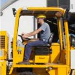
Cabin Open cabin FOPS with 180° swivelling driving post, high sitting position for improved visibility. 4 working lights for moving in tunnels.
